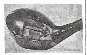
The photograph above is a close-up of a new golf club fitted with an impact indicator device which enables a golfer to gauge the force behind his stroke. The disc on the side of the club is the head of a piston which absorbs the impact of a golf ball against the club and causes the pointer to move across the calibrated scale. The device was invented by Dr. Michael J. Plese, a dentist in Amityville, L. I.
