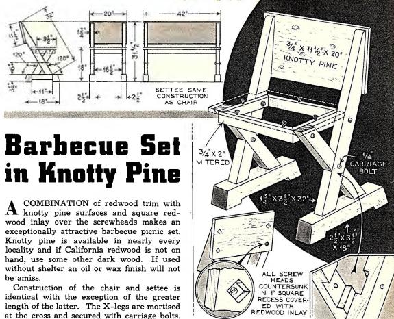
Construction of the chair and settee is identical with the exception of the greater length of the latter. The X-legs are mortised at the cross and secured with carriage bolts. Lag screws are inserted up through the bottom of the feet. Knotty pine is used for seat and back, and a square recess about ½-inch deep is chiseled for each screwhead, then inlaid with redwood.
