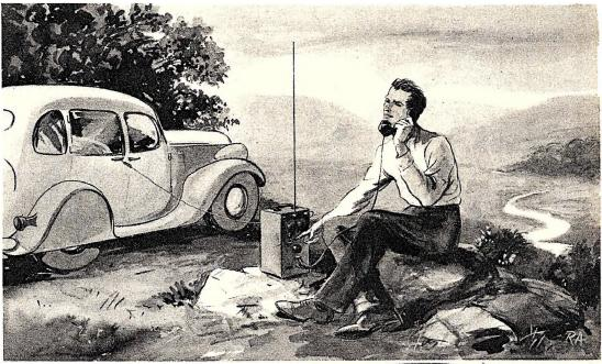
Five-meter transmitters and receivers operate beat at high altitudes with no intervening objects between communicating stations. Inasmuch as this rig is selfcontained, it can be used in car during summer trips.
