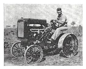
Constructed from old auto and tractor parts by Herbert H. Groom, this tractor boasts five forward and four reversespeeds.
