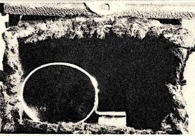
FOCUSING AID FOR GRAFLEX OWNERS. A spectacle lens soldered to a small hinge and bolted to the inside of the hood will make focusing considerably easier for those whose eyes are weak or defective. This is especially useful when small stops are used or critical definition is desired. When camera is closed, it folds down against inside of hood.
