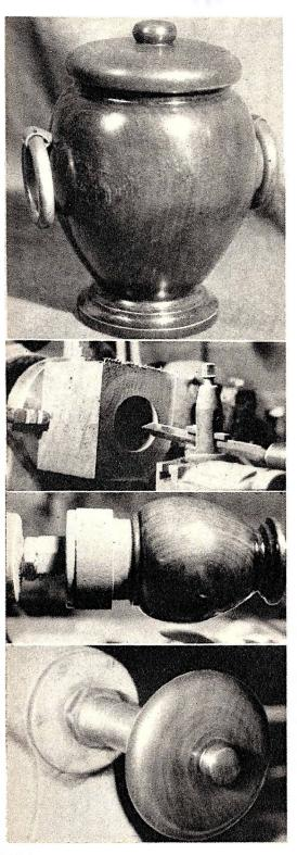
THIS walnut box can be constructed in an evening and is useful as well as attractive when completed. If a metal turning lathe is available the inside turning is done on it, to good depth, accurately and easily.
