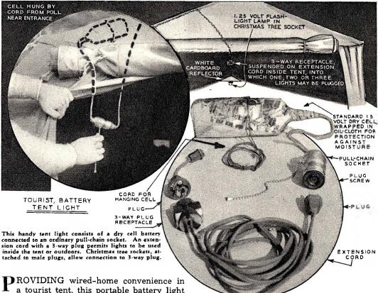
PROVIDING wired-home convenience in a tourist tent, this portable battery light can be switched on or off from outside the tent by reaching through flap and pulling chain of a pull-chain socket. From inside, the chain may be more easily located in the dark if the pendant has been coated with luminous paint.
