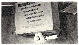
A small electric hair drier can be used to heat a paint drying cabinet as shown in the photograph. The "cabinet" can be nothing more than a cardboard packing box. A hole should be placed in the bottom to permit the air to circulate.
