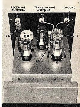
The layout of parts shown by this rear view should be followed as closely as possible for best results. The transmitting tank coil is located at the right.
