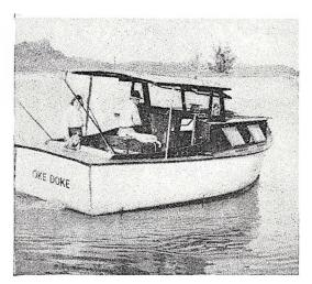
Built to MI plans by A. L. Chase and powered by a converted auto engine, this 25-foot cabin cruiser travels 14 m. p. h.
