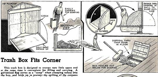
A pivoted trash container shown at upper right is arranged so that it will swing outward through an opening in the wall. It can be dumped from the outside, and in either position closes the opening against flies and drafts. If the shop floor is slightly higher than ground level, a box can be pushed under a trap door, and all rubbish can be pushed into it. The box should be provided with a small handle.—Hi Sibley.
