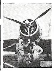
The photograph shows one of the new hydromatic propellers in full-feathering position, showing how blades are feathered to stop "wind-milling" during flight with engine not operating.
