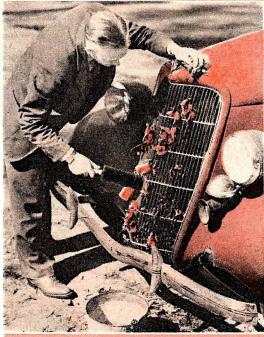
Fins or air passages stopped up with mud, insects or leaves; bent or loose baffle plates, tubes or passages pinched or bent all serve to overheat an engine. Clean the radiator cores with a brush or air hose. Don't attach license to the grille.
