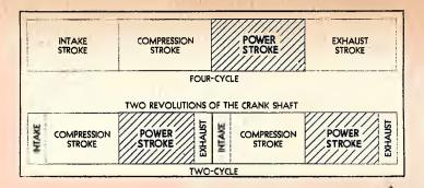
ward stroke as in a four-cycle engine. Thus if the power stroke in a two-cycle engine is made as efficient as the power-stroke in the four-cycle engine, only half as many cylinders are required for the same result. By operating on the two-stroke cycle it is not possible
