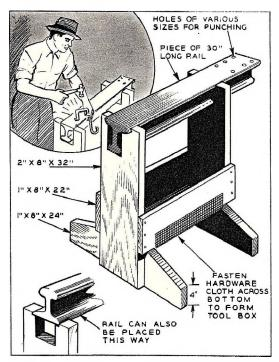
A short piece of street car rail becomes a very satisfactory anvil when mounted as shown in the drawing. The mounting is a convenient type for moving from one place in the shop to another. If its location is to be permanent, a concrete base should be used. The frame will be considerably more rigid if each of the joints is wiped with strong wood glue before they are nailed together.—L. W. Harazim.
