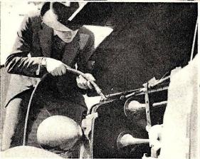
Above—When checking radiator watch for insufficient water supply, obstructed flow, anti-freeze not removed, leak in overflow pipe, pinched overflow pipe, inside of tubes or passages clogged. Left—Radiator should be flushed. A garden hose will answer the purpose. Disconnect the hose between radiator and engine when flushing the former.
