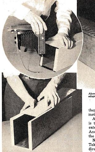
Circle—The camera is turned upside down, and slid over the metal runners. The outfit can be used vertically, as shown on preceding page, or turned on its side if the subject is wider than it is high. Above—Before nailing on the top, paint entire inside of box with flat black paint, to kill internal reflections.
