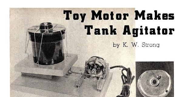
Above: The completed agitator with the loaded film tank in place. Right: Close-up of the rocker cam, made from a small pulley, about an inch in diameter.
