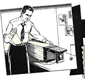
THE usual way to make close-up pictures of small objects is to insert a speciallymade tube between the camera and the lens. Since most cameras have their lenses permanently attached, this procedure is not
