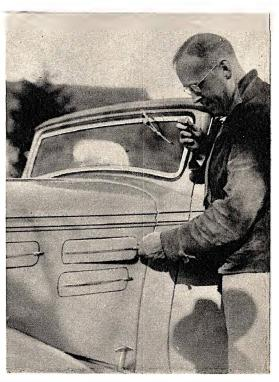
Much overheating is due to failure to open hood louvres. These allow exit of the hot air after it cools the engine.
