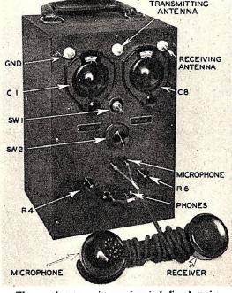
The complete transmitter-receiver including batteries is contained in a single metal cabinet. The microphone and receiver is shown in front.
