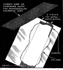
If solder refuses to stick when soldering perpendicular seams, a narrow strip of screen or hardware cloth placed across the seam, as shown in the drawing, will solve the problem. When exposed to the weather, the screen will expand or contract according to the temperature, thus eliminating the possibility of cracking.—R. A. Scott.
