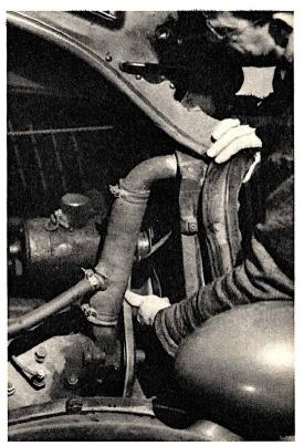
The fan belt should have about an inch play. If it's too tight the fan bearings will be cramped—and heat-up.
