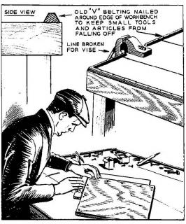
Ball bearings, small bolts and nuts, and other small articles have a tendency to roll off the workbench, falling to the floor to be stepped on, or lost. An old "V" fan belt tacked to the edge of the bench will prevent this from happening, and at the same time will not interfere with work. The narrow edge of the belt should face inside.—W. C. Wilhite.
