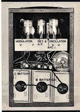
Small size batteries should be used for "B" power. Because the tubes used have comparatively low plate current drain, the life of the batteries will be long.
