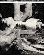
The dimesions given above are for the goblet shown in the lathe. The sharpened tang of a flat wood file makes an excellent cutting tool for scooping out the center. When the shaping is completed, the goblet is sanded while still in the lathe. If the goblet is to be used, it should be finished with several costs of varnish.
