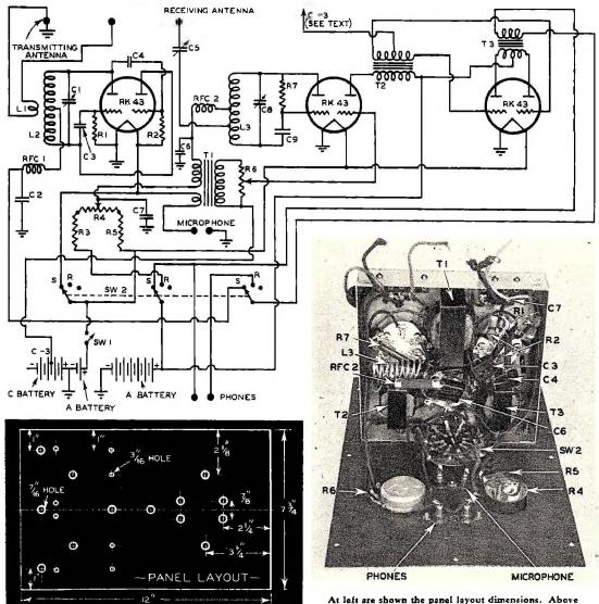
At left are shown the panel layout dimensions. Above is the layout of the parts, looking up under the chassis. The change-over switch (Sw2) is in center of panel.
