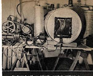
Confronted with an infantile paralysis epidemic in remote Juneau, Alaska, and unable to secure a commercially-made respirator, Dr. R. Coffey constructed an emergency "iron lung" device (above) from a large garbage can and motor-driven compressor.
