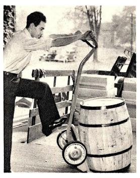
THIS all-metal drum or barrel truck requires a minimum of effort to handle heavy loads safely and quickly. Rugged all-steel welded construction insures ability to stand up under hard use. Wheels are ball bearing, steel or rubber tired.
