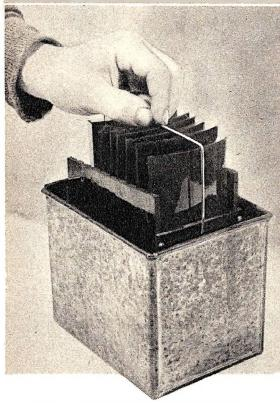
Above: The rack loaded with film, about to be lowered into the developing tank.
